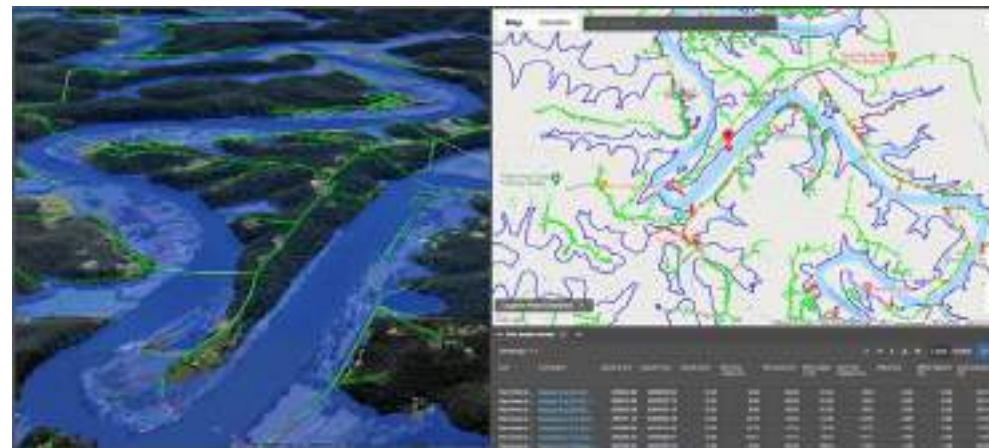
A Neara dashboard used by Endeavour Energy to prioritize their emergency response and recovery efforts. The dashboard integrates live river depth readings, historic flood maps, and dynamically calculated flood polygons to identify assets at risk of water contact.
