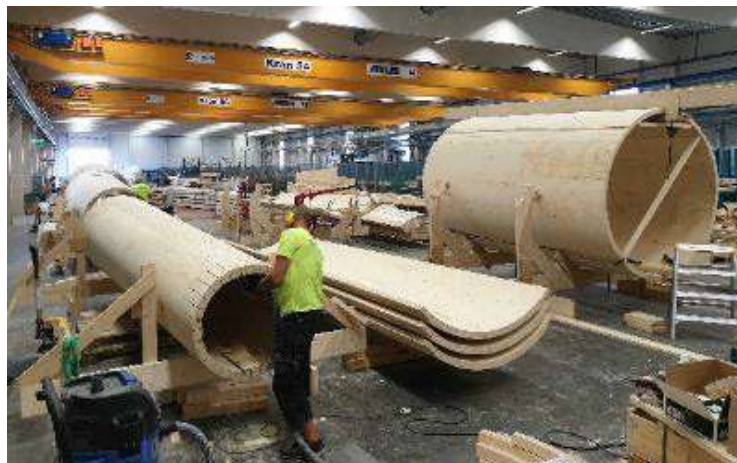
Figure 26 Manufacturing of the 30m Modvion prototype tower
