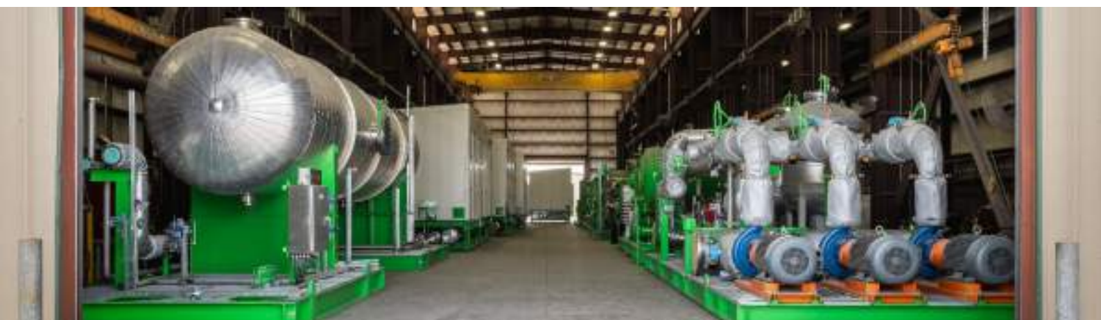
Roadrunner | Assembled HYPRPlant skids for Roadrunner awaiting shipment to project site| image provided by Electric Hydrogen
