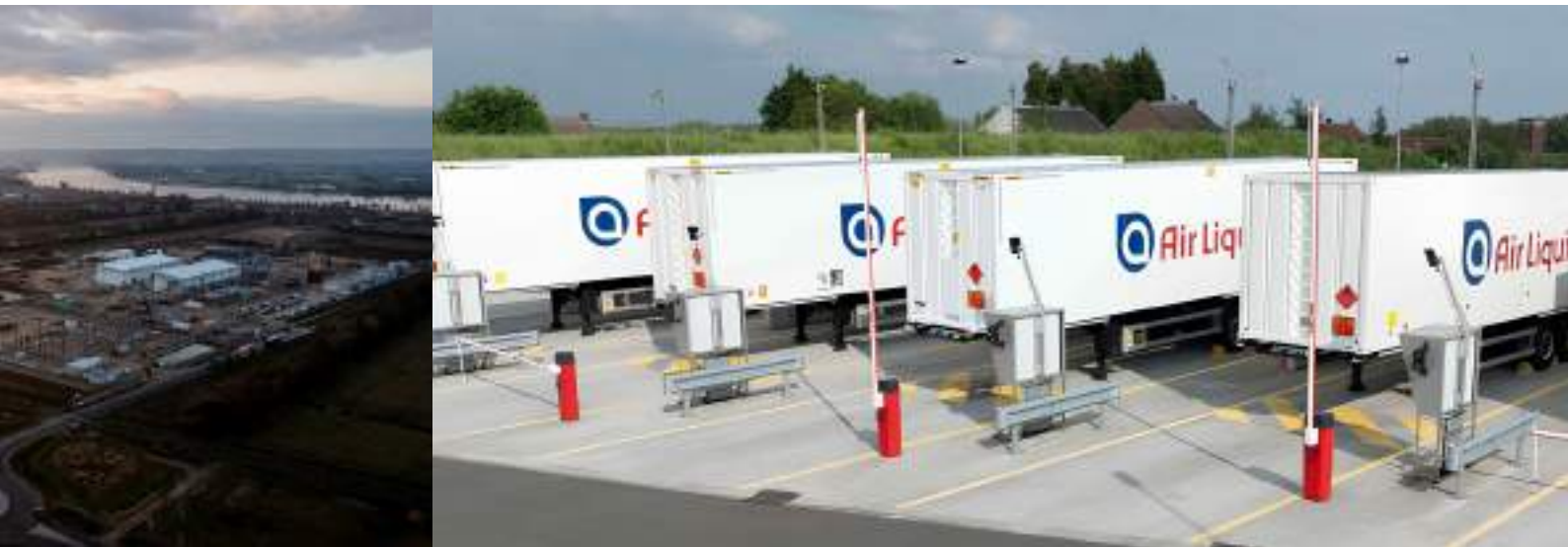
Normand'Hy | Aerial view of Normand'Hy plant and 300bar hydrogen trailers | images provided by Air Liquide
