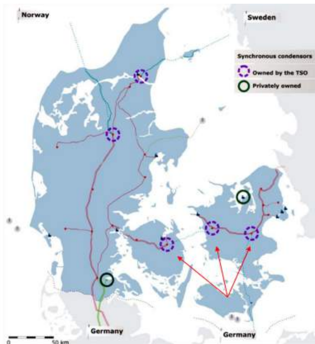
Figure 4.3 Locations of synchronous condensers in Denmark
