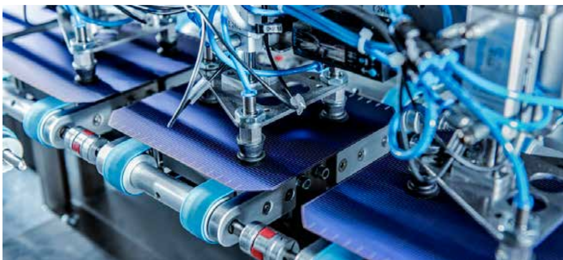
Fig. 6 - Leverage for cost reduction lies in increasing efficiency of modules, the reduction of material costs and high module reliability. An industrial R&D project within the framework of a European cooperation ( SOLAR-ERA.net ) has made significant contributions to these challenges by combining fine-line metallization of solar cells with the cell connection technology from Meyer Burger. On the cell level, silver paste consumption for metallization could be lowered to 5 mg/Watt, which is far ahead in the photovoltaic technology roadmap. With the modules built and tested with this approach, the total module power exceeded by 15 watts compared to commercial 3 busbar modules (Photo: Meyer Burger).
