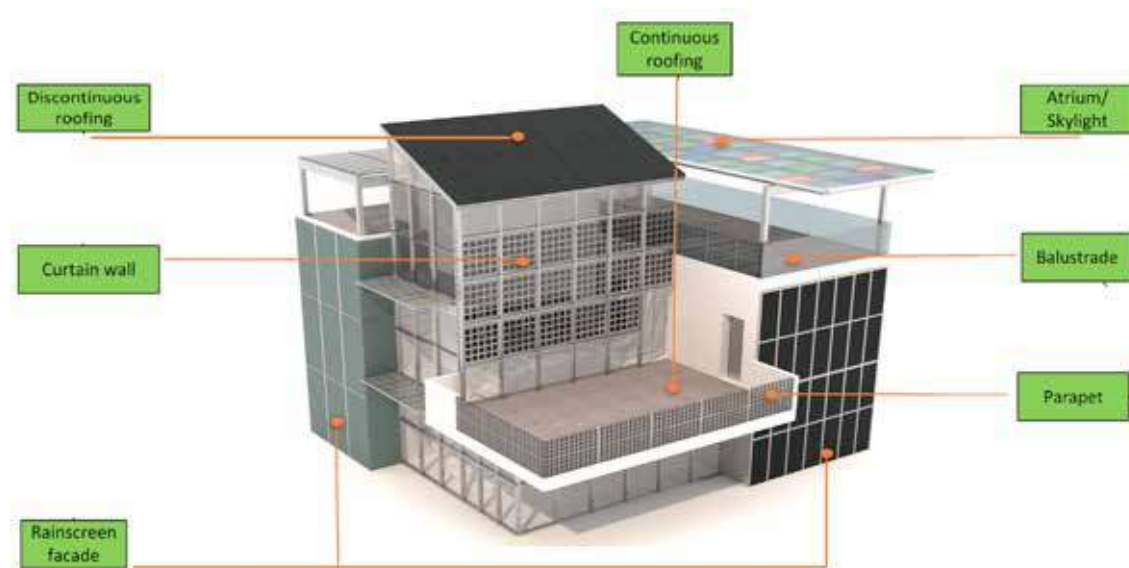
Fig. 1 - Illustration of BIPV installation scenarios categorized in activity B.2. (Source: SUPSI).
