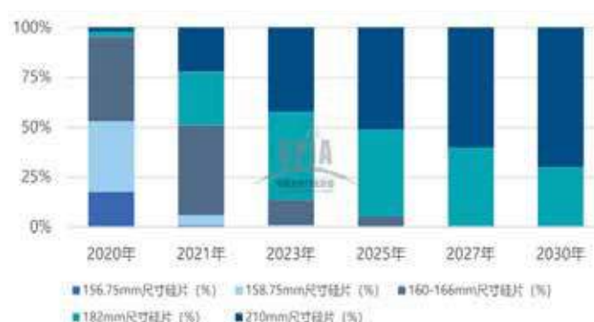
Fig. 6 - Trend of silicon wafers with different sizes.
